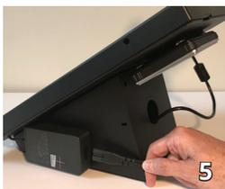
**If you need to move the device temporarily to a new location for fingerprinting, you can unplug the power cable and use battery power for up to 3 hours.**
